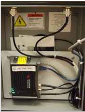
CONTROLLER SUPPLIED WITH 4G ANTENNA (EITHER TWO DIVERSITY OR ONE CENTER MOUNT - MIMO)
